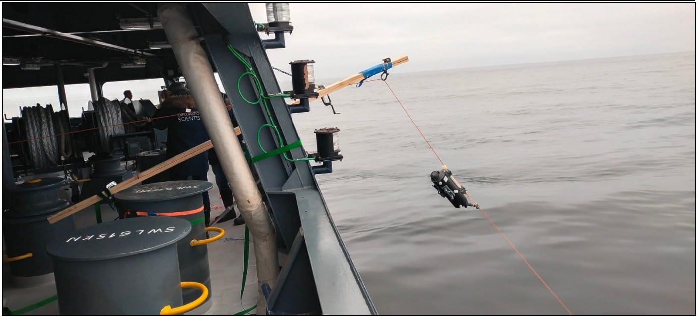
Figure 5: Deployment of a Niskin bottle from the aft of the ship to get water samples from a depth of 30 m.
