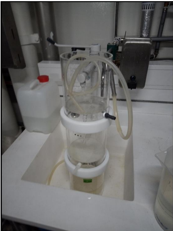
Figure 3: Continuous toxin sampling from the peristaltic pump. The water was directed to a filter tower with a tube.
