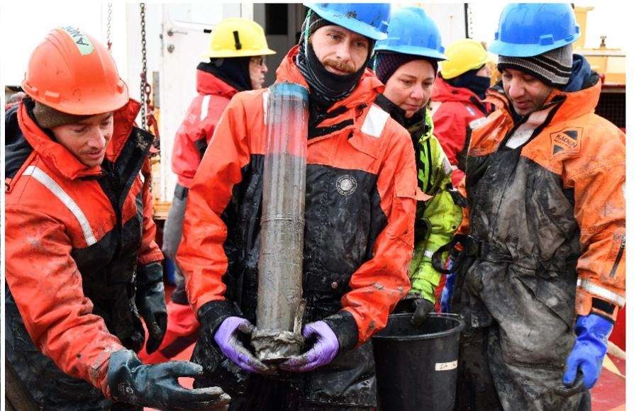
*Multicorer comes up on deck and cores get secured for further work in the laboratories. Photos: Liam Jasperse.*
