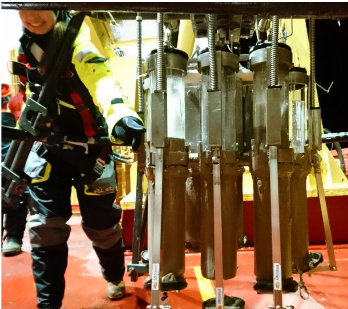
The multicorer is back on the deck and brought us eight (no seven – one core slid out) beautiful cores full of mud from the sea floor.
